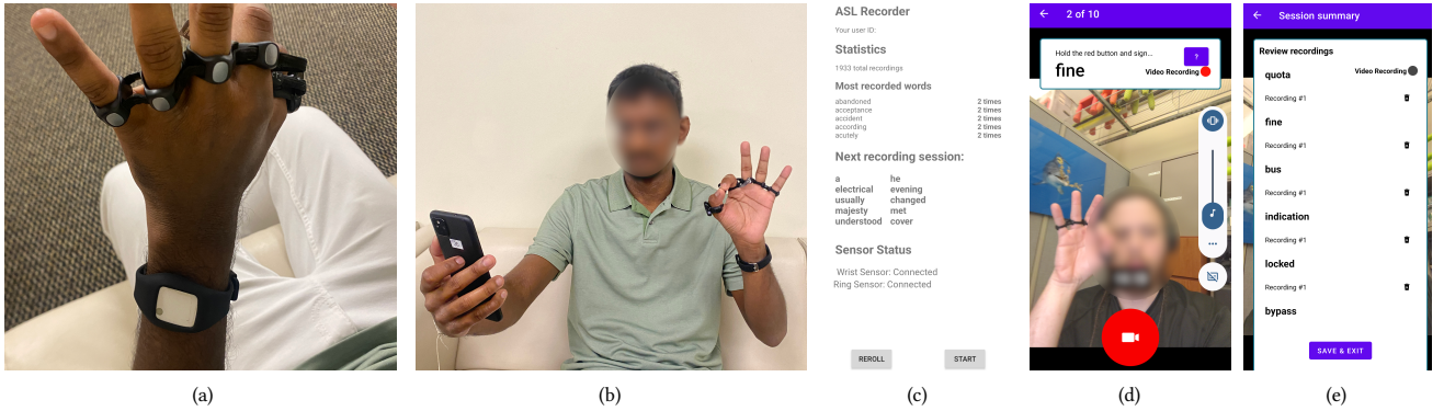
Figure 1: Overview of our data collection process using ring sensors and push-to-sign collection app. (a) Participant wearing the sensors. (b) Participant collecting finger spelling data. (c) Statistics page providing key data collection statistics. (d) Recording page where participants hold down the recording button while fingerspelling the specified word. (e) Summary page enabling participants to view and delete recordings.
