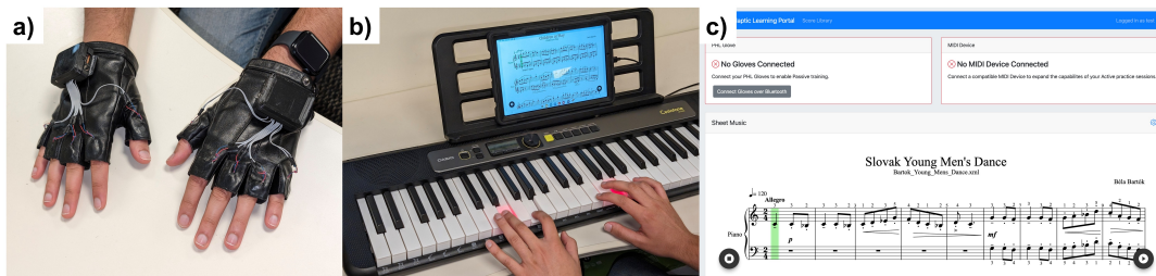
Fig. 1. a) Haptic gloves for daily passive haptic rehearsal. b) Practicing piano with our piano education system and a Casio keyboard. c) Online learning portal of our piano education system.
