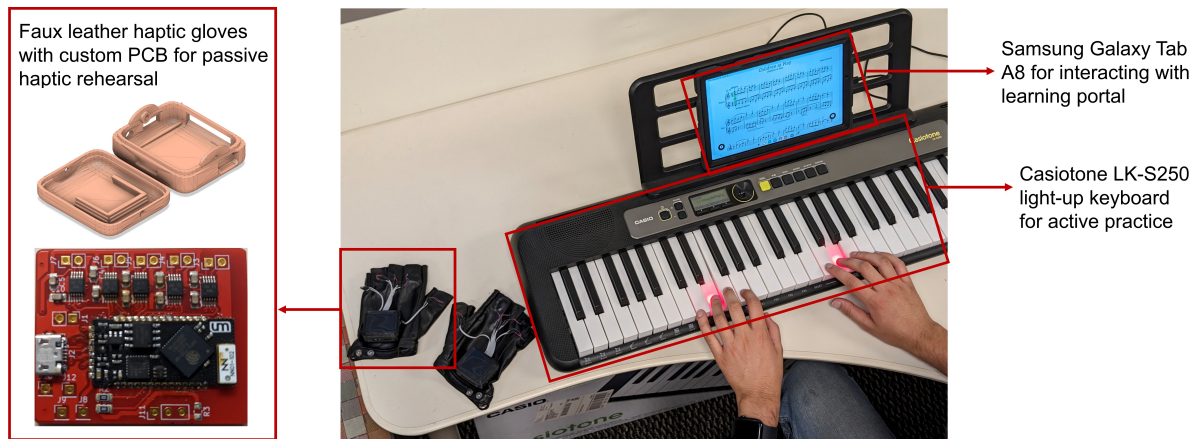
Fig. 2. Apparatus taken home by participants during study, including custom haptic gloves, Samsung Galaxy Tab tablet and Casiotone LK-S250 piano keyboard.
